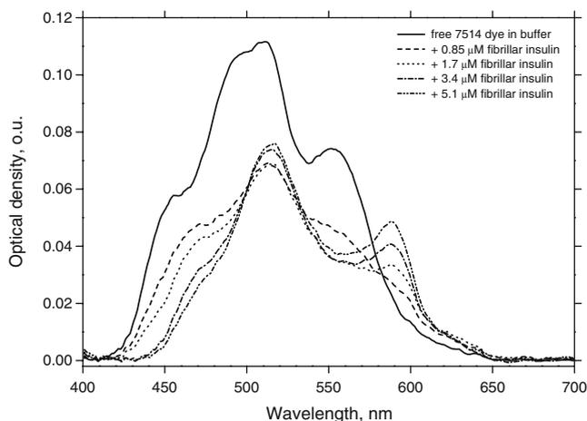
**Fig. 5** Absorption spectra of 7514 ( $5 \times 10^{-6}$  M) in free form in TRIS-HCl buffer, pH=7.9 and in presence of fibrillar insulin (0.85–5.1  $\mu$ M)
