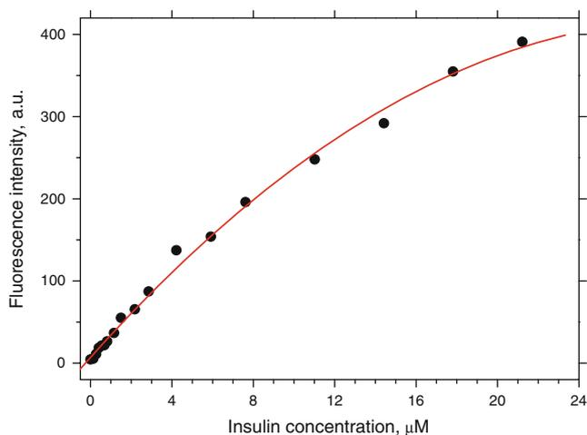
**Fig. 4** Dependence of fluorescence intensity of cyanine 7519 ( $5 \times 10^{-6}$  M) on the fibrillar insulin concentration (in TRIS-HCl buffer, pH=7.9)
