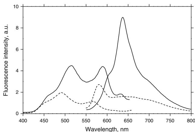
**Fig. 7** Fluorescence excitation (*left*) and emission (*right*) spectra of 7514 ( $5 \times 10^{-6}$  M) in free state in TRIS-HCl buffer, pH=7.9 (*dash*) and in presence of 1.7  $\mu$ M of fibrillar insulin (*solid*). Fluorescence emission was excited at 515 nm, fluorescence excitation spectrum was registered for 670 nm emission
