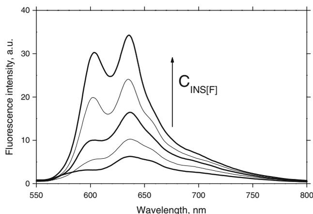
**Fig. 9** Fluorescence emission spectra of 7514 ( $5 \times 10^{-6}$  M) in presence of different fibrillar insulin concentration (0.85, 1.7, 3.4, 5.1 and 6.8  $\mu\text{M}$ ) excited at 515 nm (TRIS-HCl buffer, pH=7.9). Arrow points the insulin concentration increase
